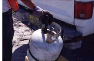
After that date and regardless of the tank's age, propane dealers **will not** refill a tank unless it is equipped with an OPD.
