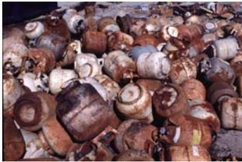
Through the Recycling Program the Solid Waste Authority (SWA) segregates the tanks, empties the propane and removes each tank valve. The SWA's commercial customers are required to pre-process their tanks prior to delivery to the landfill processing area.
